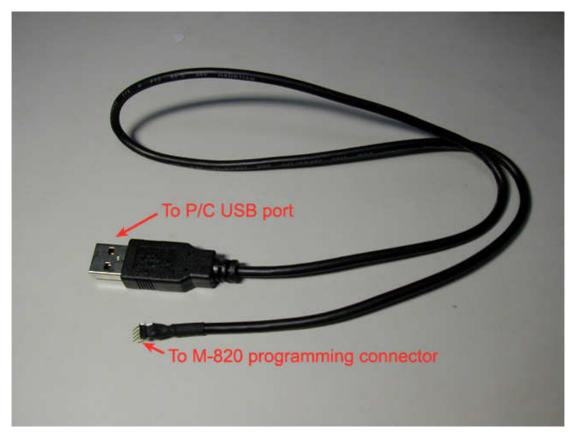
2). Insert the USB programming cable into the M-820L set
